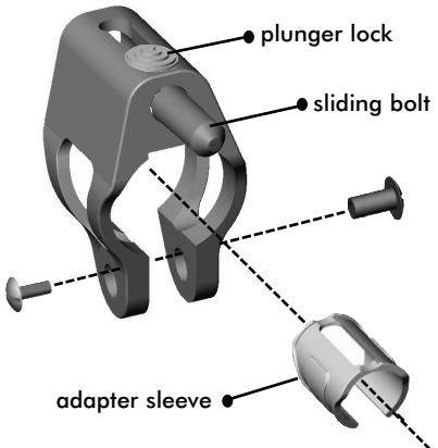
The **DuraClip** is a “lock and release” device designed to secure the drop hooks from a wheelchair (drop-base) cushion onto the wheelchair seat frame/tube. By engaging the plunger lock mechanism, the sliding bolt holds the drop hook (seat) in place; By retracting the plunger lock, the seat can be easily removed for wheelchair transportation.
